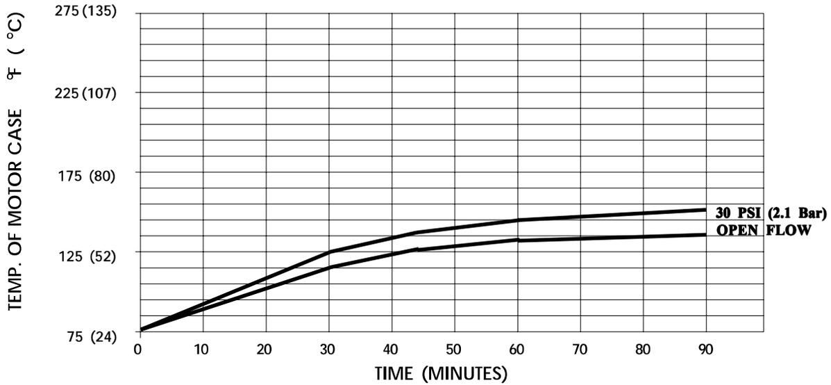
THIS GRAPH IS FOR USE AS A DESIGN GUIDE. IT IS BASED ON RUNNING CONTINUOUSLY WITH AN AMBIENT TEMPERATURE OF 75° F IN STILL AIR. THE THERMAL BREAKER WILL OPEN WHEN THE CASE TEMPERATURE REACHES 290° F.
